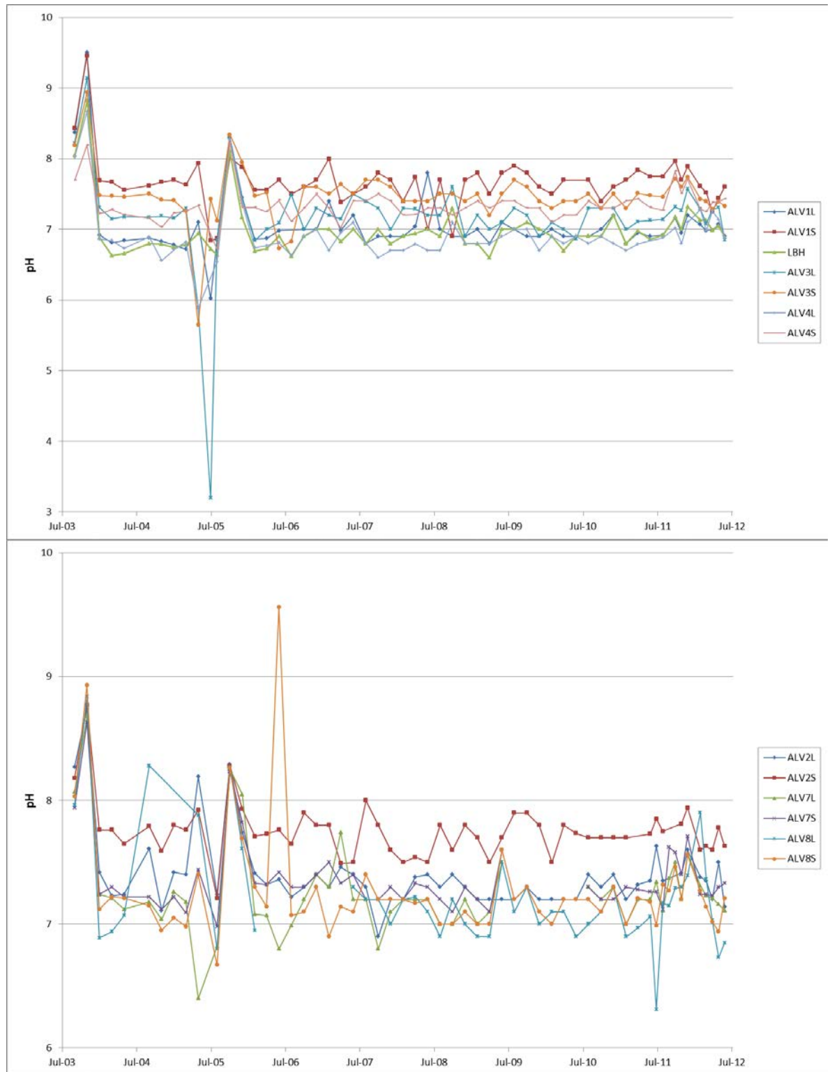
■ Figure 2-18 – pH Data for Piezometers Targeting Alluvium and Shallow Bedrock
