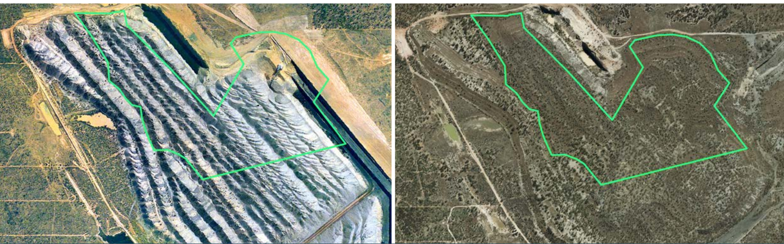
The Grasstree pit at Oaky Creek during mining and after rehabilitation. The green outline shows the area signed-off by Government.
