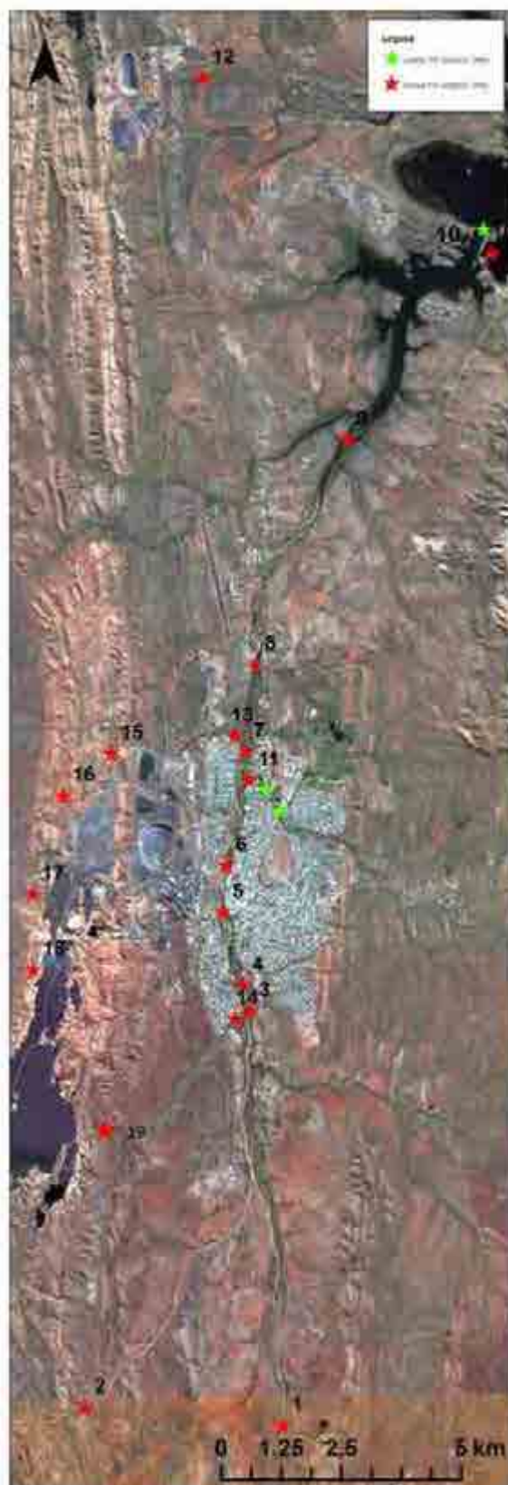
Figure 24. Summary of sites exceeding trigger values for arsenic, cadmium, and lead for 95% freshwater species protection (refer to Table 32 for site names). TV has been adjusted to the site-specific conditions of water hardness
