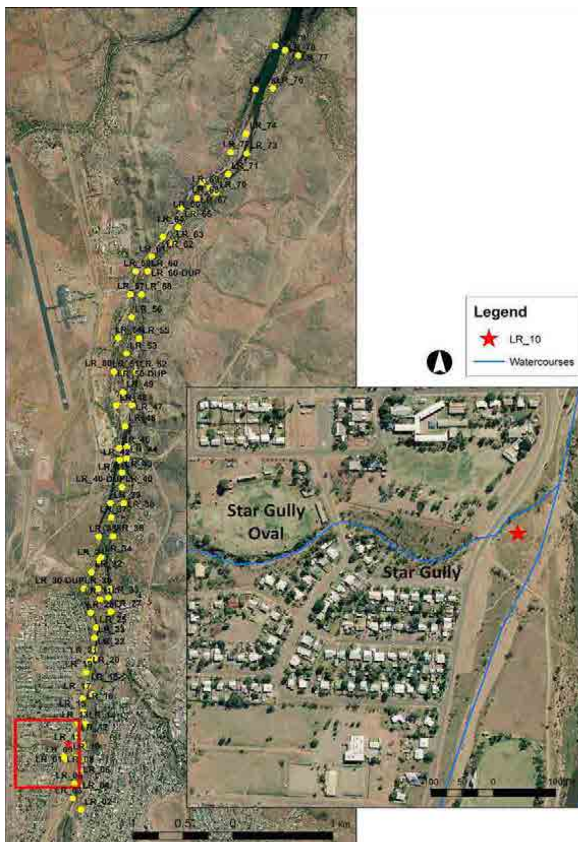
Figure 31. Sampling sites of Leichhardt River Verification Program (13-14 November 2009). The insert map shows the LR10 site, where the concentration of arsenic exceeded ISQG-Low. LR10 is identified as being contaminated for human health
